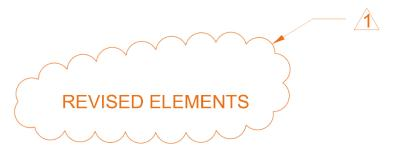
f. The "REVISIONS" block of each sheet that is changed by a revision must be completed to document the plan changes. The "REVISIONS" block should contain the addendum number inside of a triangular shape in the lower center of the block followed by the date and a brief description of the change. As the revision block fills, the oldest entry is removed from the border and placed below and outside of the printable area.
