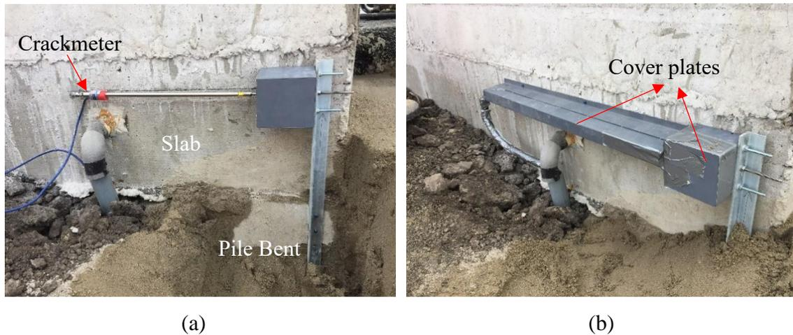
Figure 3.10 (a) Installation of NW displacement transducer (Arlington Heights Road); (b) Cover plates of NW displacement transducer (Arlington Heights Road).
