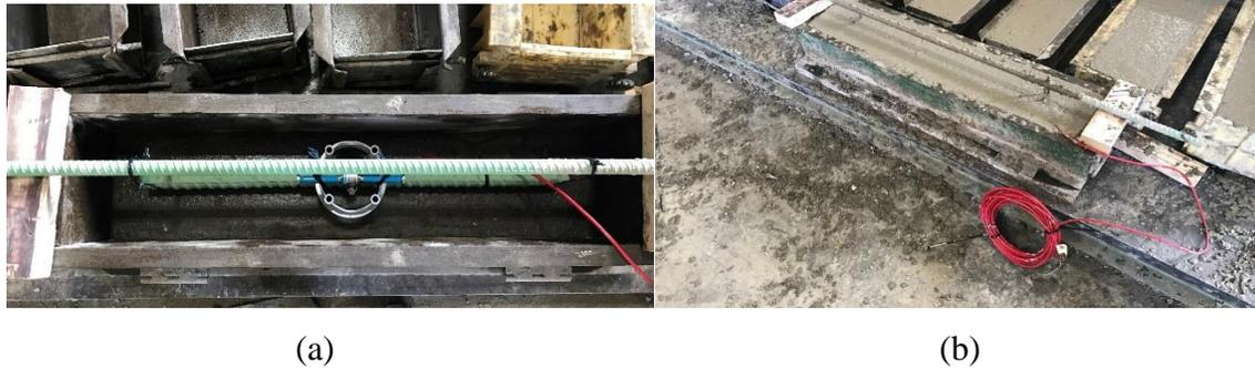
Figure 3.8 (a) Temperature beam with embedded gage and reinforcement bars; (b) the temperature compensation beams being cast.
